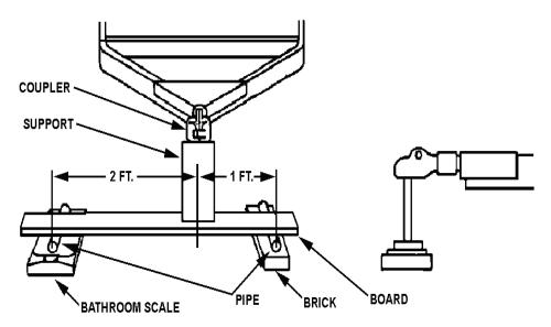
Lower the tongue until the coupler rests on the block support and the jack is ½ inch above the ground. The scale reading, minus the weight of the block support is the tongue weight.
