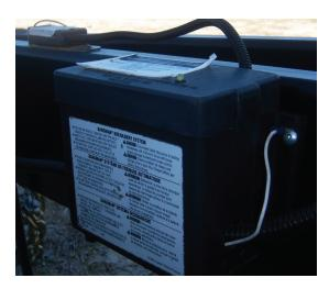
Connect the pullpin lanyard to the tow vehicle so that the pullpin will be pulled out before all of the slack in the safety chains is taken up (see Breakaway Brake System figure). Do **not** connect the pullpin cable to a safety chain or to the hitch ball or hitch ball assembly. This would keep the breakaway brake system from operating when it is needed.
